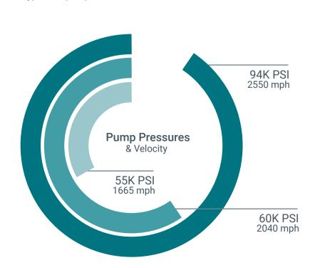
The higher the pressure, the more parts cut - resulting in lower cost per part.
